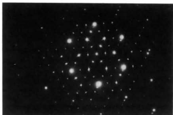
Fig. 2. SAED pattern taken from the plane-view specimen showing a pseudo-sixfold rotation symmetry.
